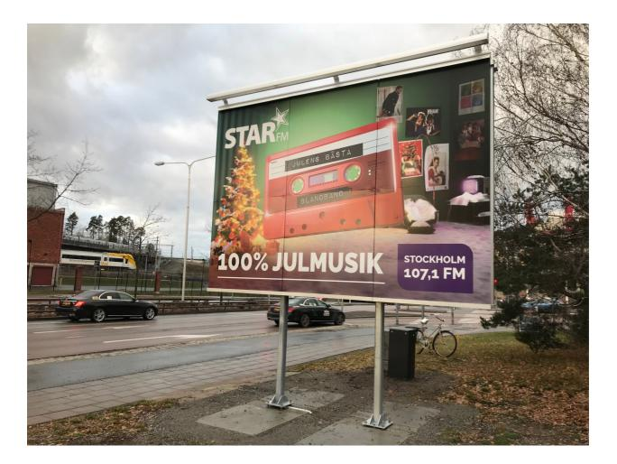
Big billboard where three separate corrugated cardboard pictures are combined together into a single large picture. The image size in combination with the board having a height of about 4500 mm means that the readability at longer distances and in environments with fast traffic is very good.
